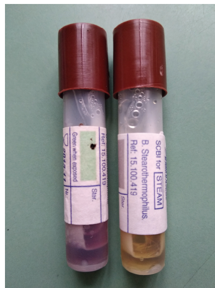
Figure 4. Biostrip method a) successful sterilization on the left; b) unsuccessful sterilization on the right
