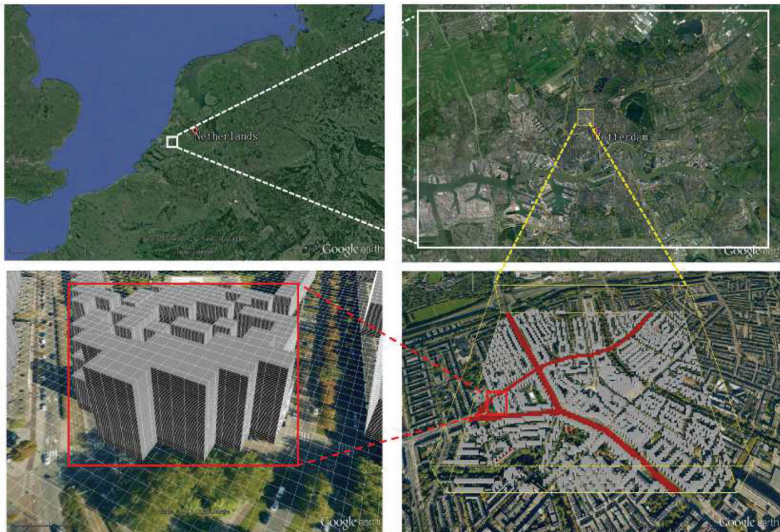
Figure 2. The simulated case is shown in the Google Earth: region (The Netherlands) scale; city (Rotterdam) scale and neighborhood (the “Oude Noorden”, 2 \times 2 \text{ km}^2 ) scale including computational mesh and blocks (~1800 blocks are included in simulations) representing parts of buildings. The emission sources (due to intensive traffic along 3 streets) are marked in red. The region within the yellow box is geometrically reconstructed and simulated in detail, Liu and Kenjeres(2017).
